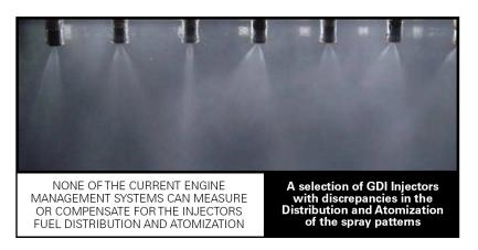
With the ASNU system, users can inspect individual fuel injectors either on a per-cycle basis or sequentially. In sequential mode, they can evaluate injector performance across a variety of simulated driving cycles programmed into the ASNU system, based on different millisecond and RPM settings. The number of injectors being tested is the only limiting factor for RPM and millisecond settings in the sequential testing operation.
