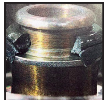
Bad Oil Rail Seal
